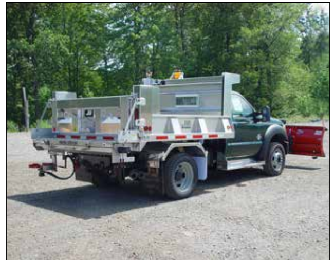
Corrosion resistant aluminum light-duty dump bodies are a favorite choice for snow and ice control applications.
